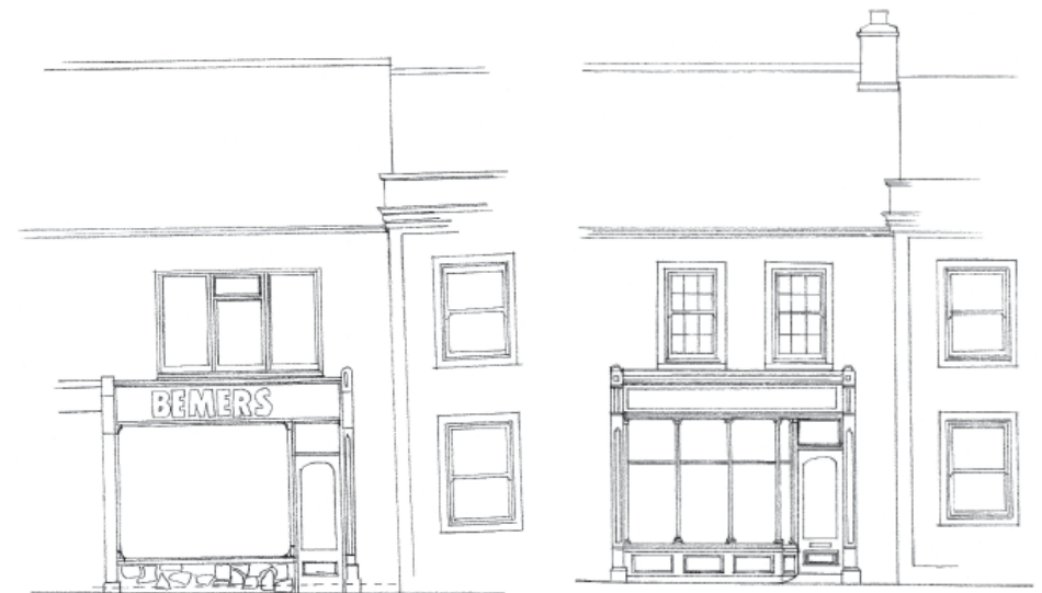
Before, modern window, missing console, missing pilaster detail, polygonal raised mortar stone work, introduces a horizontal emphasis
